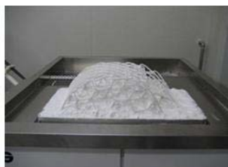
圖 2-13 selective laser sintering SLS
