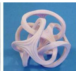
圖 2-14 laminated object modeling, LOM
