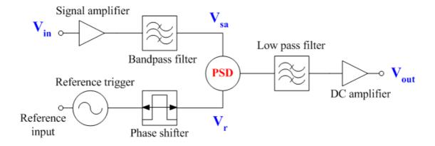
Fig. A Functional block diagram of a lock-in amplifier.
