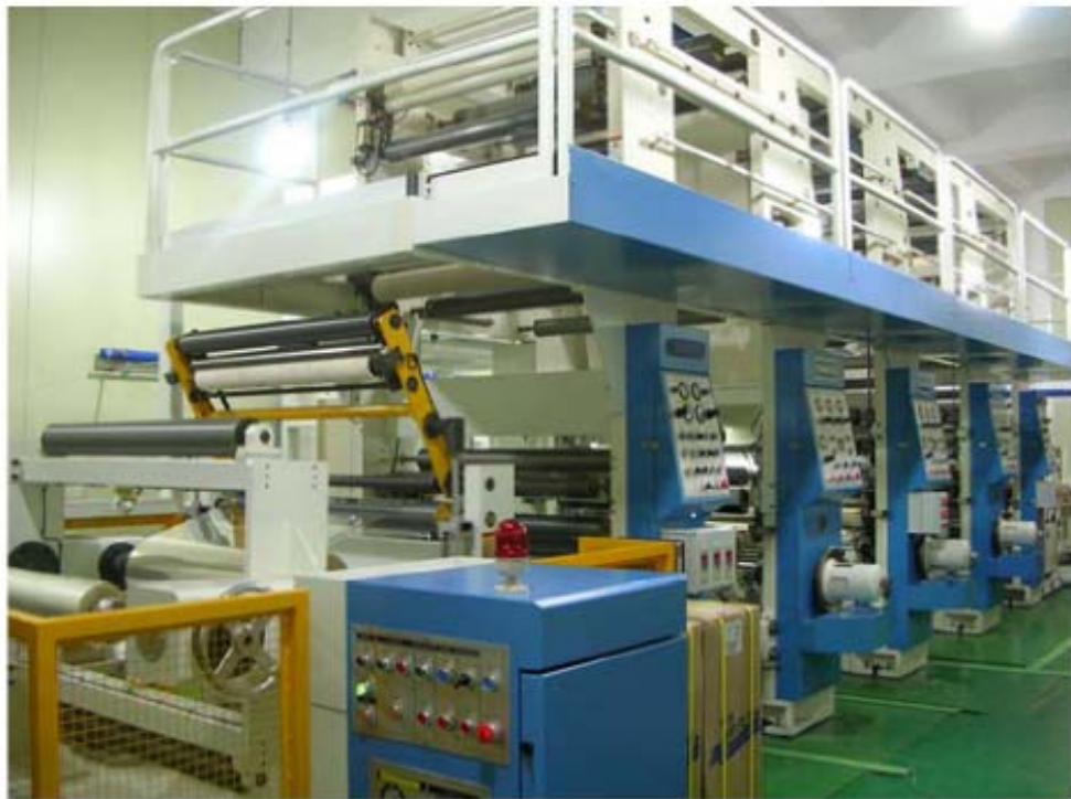
Figure 1-9. Actual gravure printing machine [15].
