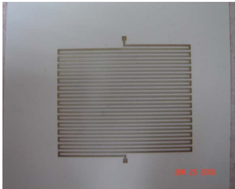
Figure 2-5. The photo of spiral line structure printing results.
