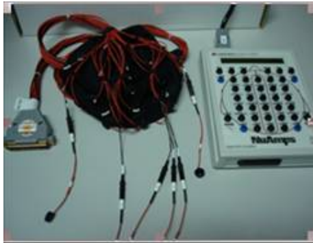
Figure 1.3: EEG measuring devices. From right to left is the EEG amplifier and the electrode cap.
