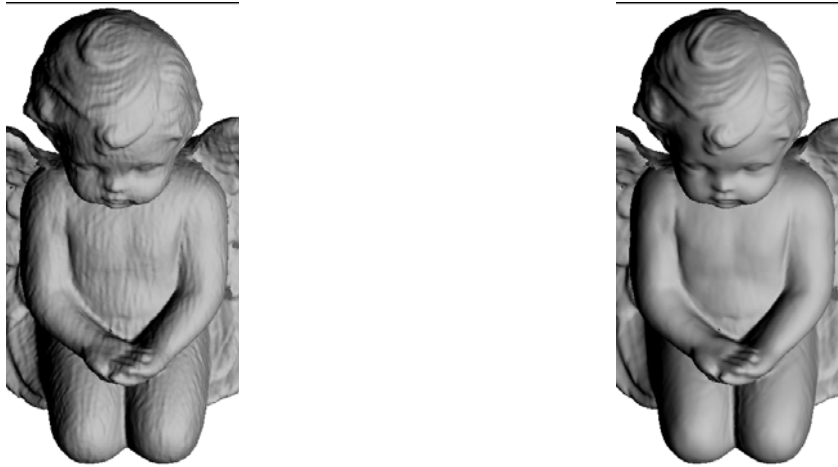
Fig.9 least square optimization. (Left) Several range scans were aligned and merged. (Right) The result was later optimized with mapped normals coming from several independent photometric stereo scans.[1]
