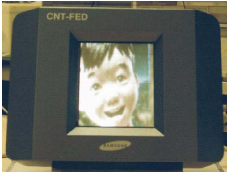
Figure 2-21 Video running image of the CNT-based FED [Chung 2002-4045] . The size of active area is 5 inch diagonal and operated in the gate electrode of 100 V and anode biases of 1.5 kV, respectively, which was observed with a duty ratio of 1/120 and a frequency of 100 Hz.
