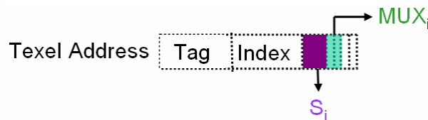
Fig. 3-9 S_i and MUX_i in address with tile size 2 \times 2
