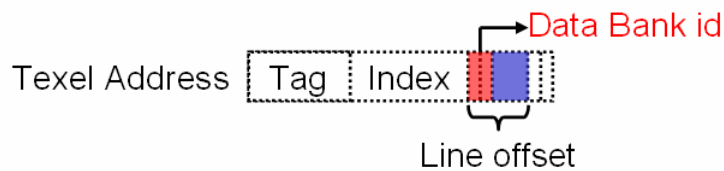
Fig. 3-3 data bank id field in address
