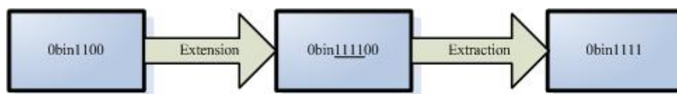
Figure 10: Right shift procedure in symbolic execution
