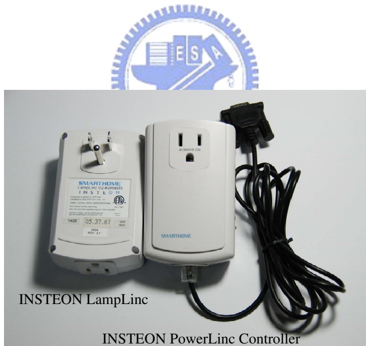
Figure 6.6: INSTEON controller and dimmer.
