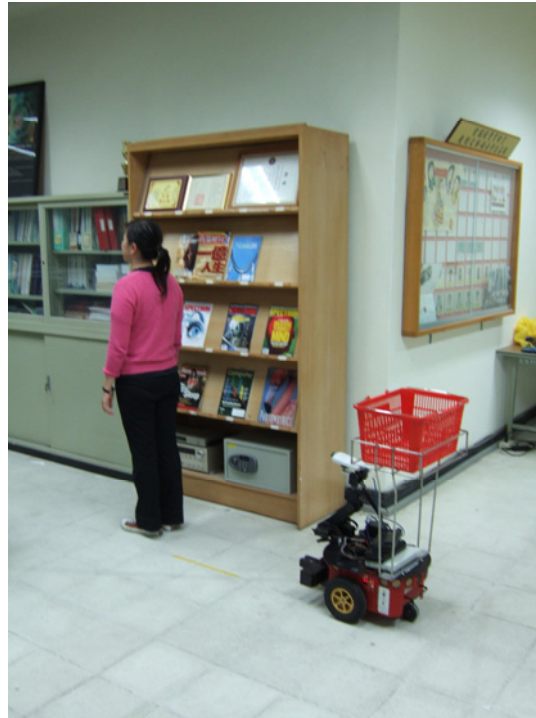
Figure 7.2 The vehicle follows a person as a shopping cart.
