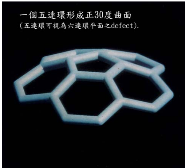
Figure 1.2 : A scheme of pentagon in a grapheme layer. Pentagons always produce a positive curvature ( 30^\circ ) of the grapheme layer [19].
