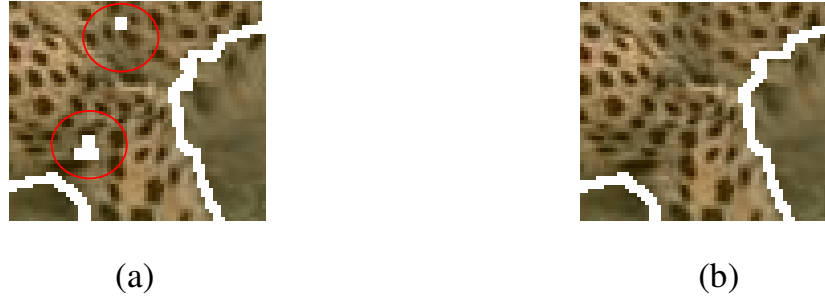
Fig. 2.5 An Example of Case 1 for fragments removing. (a) The enlarged partial result in Fig. 2.4(b) with two fragments circled by red color. (b) The result after removing two fragments in (a).
