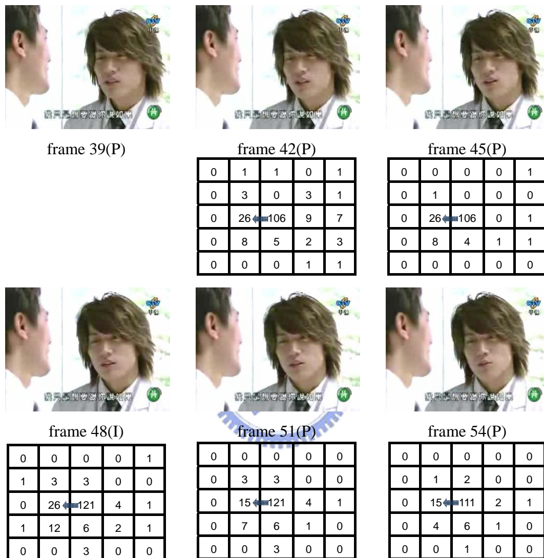
Fig. 5-6. Object movement and the corresponding OMMs.
