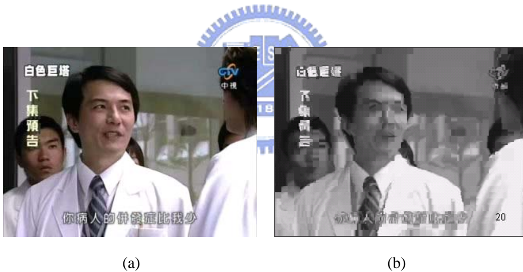
Fig. 2-2. Intra frame prediction. (a) Original frame.(b) Predicted Luma part of (a).
