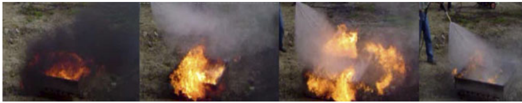
Figure 6. Pictures of Class B (pan fire) fire test.
