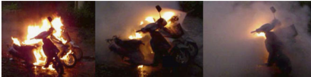
Figure 7. Pictures of motorcycles fire test.
