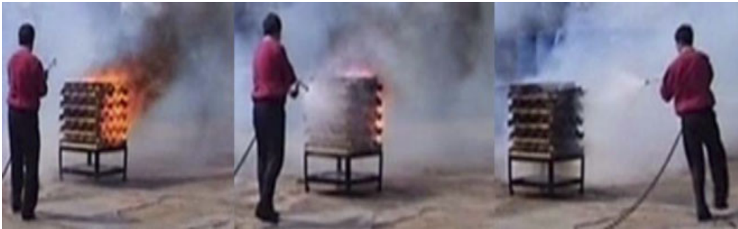
Figure 5. Pictures of Class A fire test.
