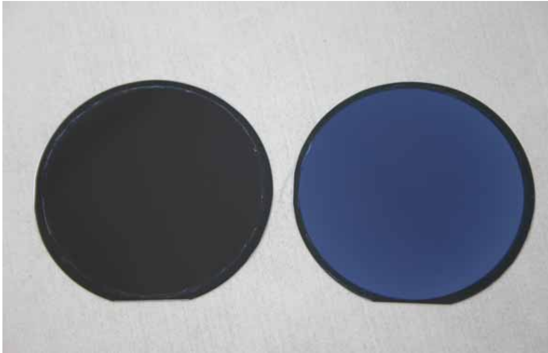
Fig 4.9 Photograph of wafers with GaAsN bulk material deposited on GaAs substrate. The wafer on the right side was grown with too high substrate temperature, the wafer on the left side was grown in the correct region temperature.
