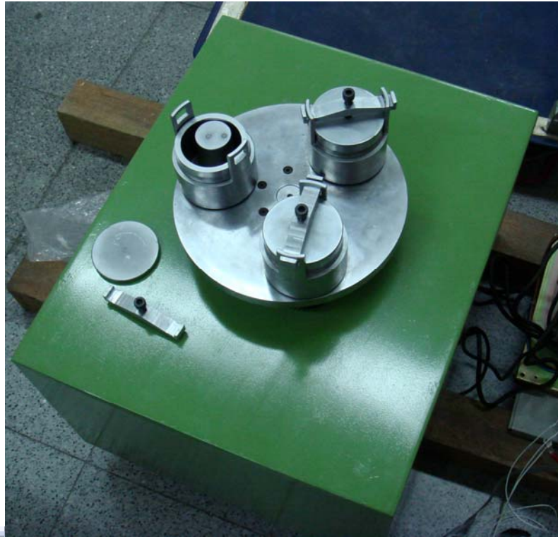
Figure 3.7 The hammer in the planetary ball mill machine
