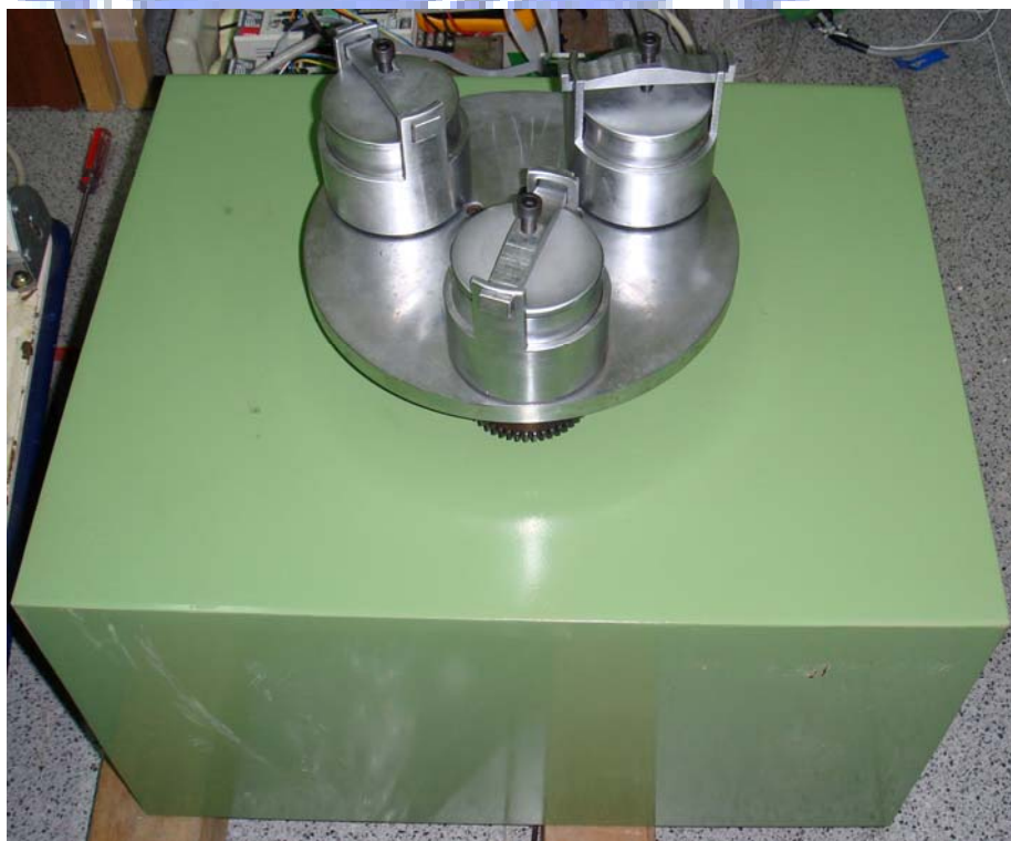
Figure 3.6 The entity of the planetary ball mill machine
