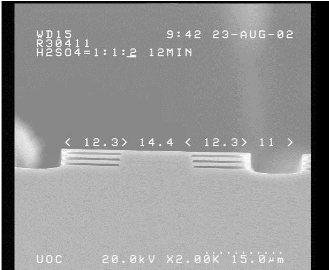
Figure 5-18 The cross section of the stable suspended InP/airgap DBRs captured by SEM.
