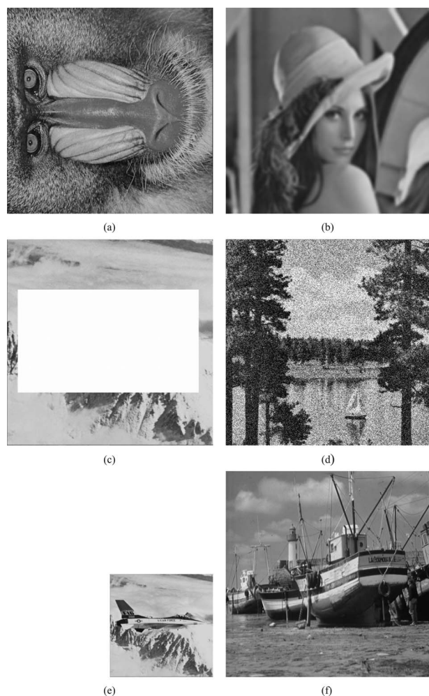
Fig. 5 Some alternations of Fig. 3: (a) the watermarked image Baboon is rotated through 90 deg; (b) the watermarked image Lena filtered by a low-pass filter; (c) the watermarked image Jet is cropped; (d) noise is uniformly added to the watermarked image Scene; (e) the watermarked image Jet is shrunk to a quarter of its size; and (f) the watermarked image Scene is completely replaced by another image Boat.
