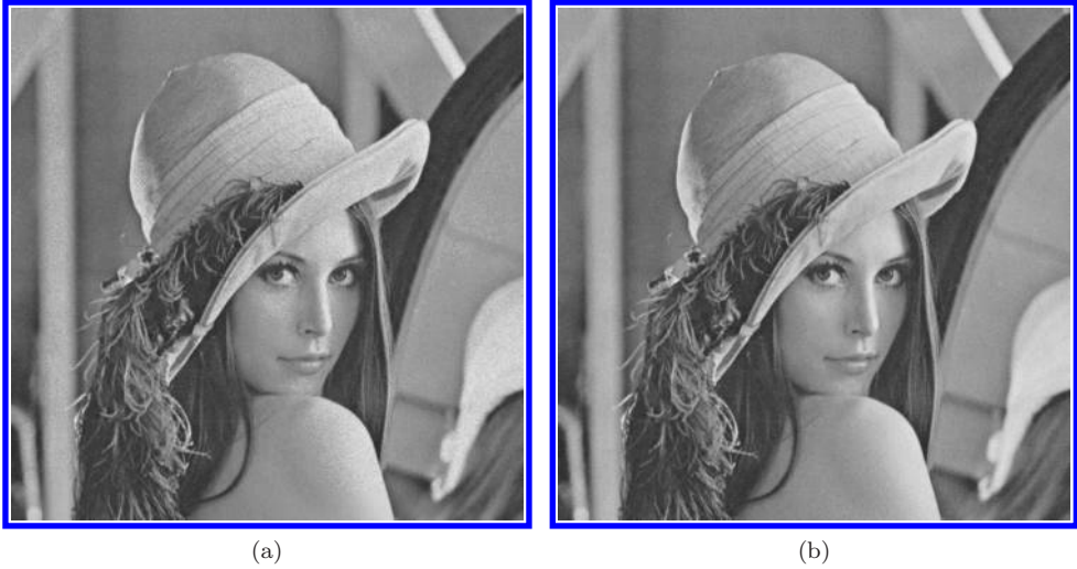
Fig. 4. The stego-images obtained by embedding a 256 \times 512 important image Jet [Fig. 6(a)] in a 512 \times 512 Lena (Fig. 5). (a) The stego-image obtained by the pixel-based method 13 (PSNR = 31.05 dB); (b) the stego-image by using our variance-based method (PSNR = 34.76 dB).
