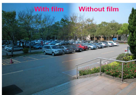
Fig. 5. Photograph taken by digital camera while the front of camera lens is with and without an optical film with the ASS surface covered with the 50-nm-thick silver layer.
