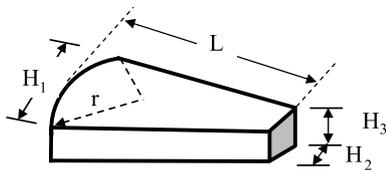
**FIGURE 2** Schematic of a lens duct, in which  $r$  is the radius of the input surface,  $L$  is the length of the duct,  $H_1$  is the width of the input surface,  $H_2$  is the width of the output surface, and  $H_3$  is the thickness of the duct
