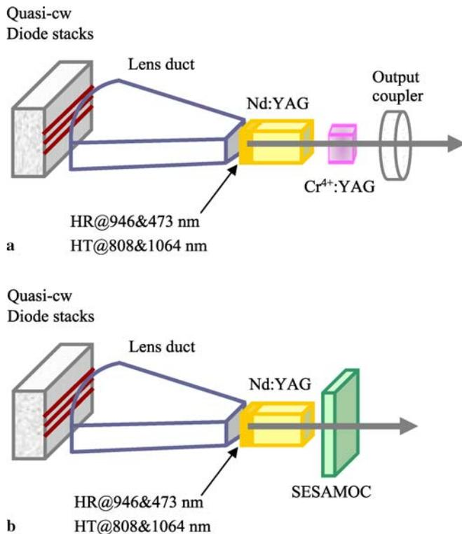
**FIGURE 1** Schematic of a diode-pumped passively Q-switched Nd:YAG laser at 946 nm: HR, high reflection; HT, high transmission. (a) with the Cr<sup>4+</sup>:YAG crystal as a saturable absorber; (b) with the InGaAs QWs as a saturable absorber and output coupler
