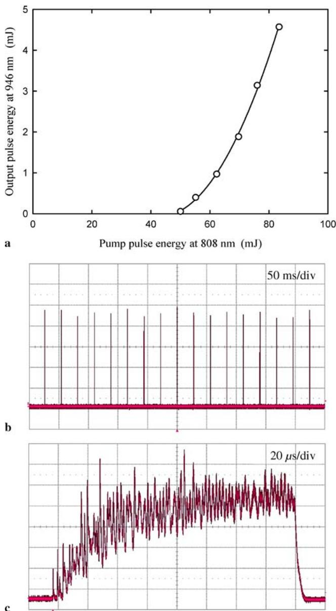
**FIGURE 4** (a) Experimental results of the free-running operation for the output pulse energy as a function of the pump energy; (b) experimental pulse train at 83 mJ of pump energy; (c) temporal shape of a single pulse
