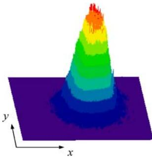
**FIGURE 7** Spatial distribution of the output beam recorded with an infrared CCD
