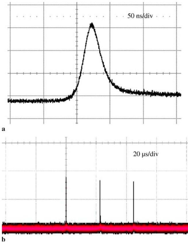
**FIGURE 6** (a) Typical oscilloscope trace of a single pulse; (b) typical oscilloscope trace of triple pulses with the InGaAs QWs as a saturable absorber
