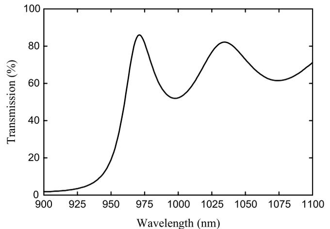
**FIGURE 3** Measured results of the low-intensity transmission spectrum for the InGaAs SESAMOC
