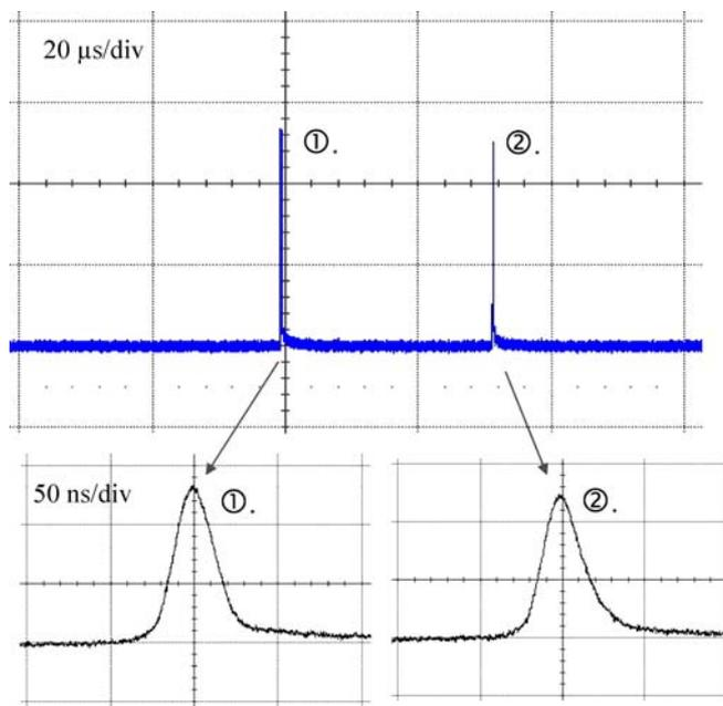
**FIGURE 5** Upper trace: typical result of double pulses in the passively Q-switched Nd:YAG/Cr<sup>4+</sup>:YAG laser at 946 nm; lower traces: expanded shape of each pulse
