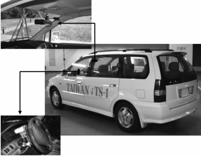
Fig. 1. TAIWAN iTS-1 with the zoom-in view of CCD and motor driver.
