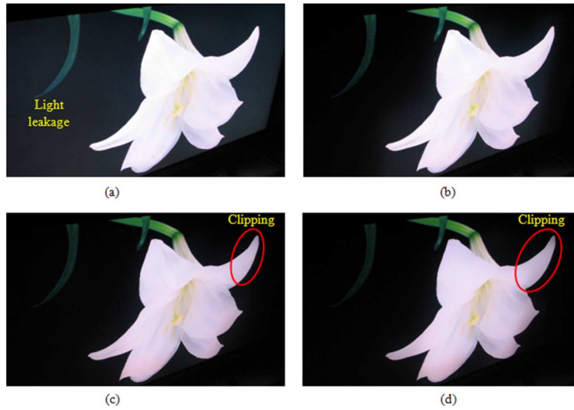
Fig. 11. Lateral pictures of a 37-in HDR-LCD by using the: (a) the full-on backlight, (b) IMF, (c) square root, and (d) average methods.
