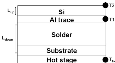
Fig. 6. One-dimensional lumped model for thermal resistance. The major heat generator is the Al trace and the Si die dissipates most of the heat.
