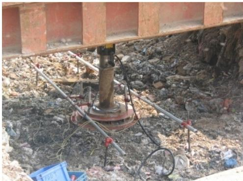
(c)位移感測計及 Load cell
