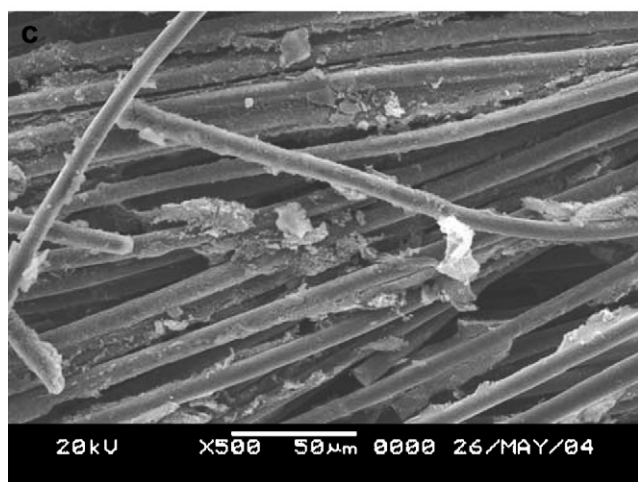
Fig. 7 – The structure of the gas diffusion layer observed using SEM (a) without chloride (b) with \text{NaCl} and (c) with \text{CaCl}_2 .
