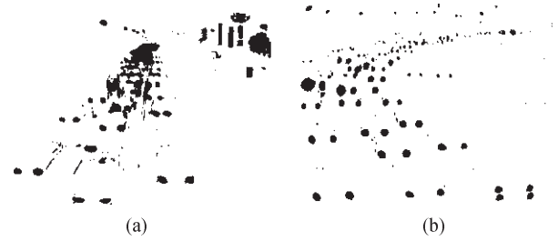
Fig. 4. Results of performing the bright-object segmentation process on the traffic-scene images in Fig. 1. (a) Lighting objects extracted from Fig. 1(a). (b) Lighting objects extracted from Fig. 1(b).
