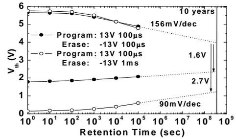
Fig.12. Retention of 10k P/E-cycled MONOS devices with 12nm
