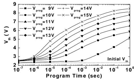
Fig.4. The measured program characteristics from  $I_d$ - $V_g$  for 16nm AIN MONOS devices. The  $L_g$  is 10 $\mu\text{m}$ .
