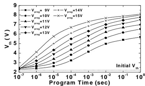
Fig.6. The measured program characteristics of MONOS with 12nm AIN.
