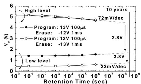
Fig.8. Retention of MONOS devices with 16nm AIN at 25°C. The P/E decay rates are only 72/22 mV/dec.
