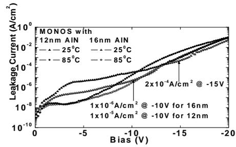
Fig.2.  $J_g$ - $V_g$  curves of MONOS memory with 12nm and 16nm AIN at 25 and 85°C. The  $J_g$  is 1 order of magnitude lower than the data from [3] due to higher  $\Phi_B$  of IrO<sub>2</sub>.
