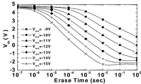
Fig.5. Erase characteristics of MONOS memory with 16nm AIN. The device was initially programmed at 13V for 100 $\mu\text{s}$ .
