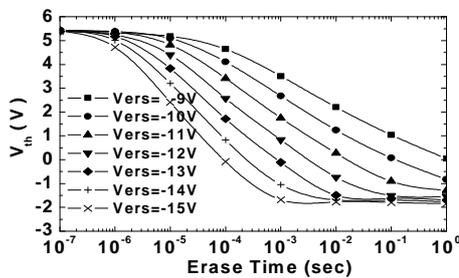
Fig.7. Erase characteristics of MONOS memory with 12nm AIN. The device was initially programmed at 13V for 100 $\mu\text{s}$ .
