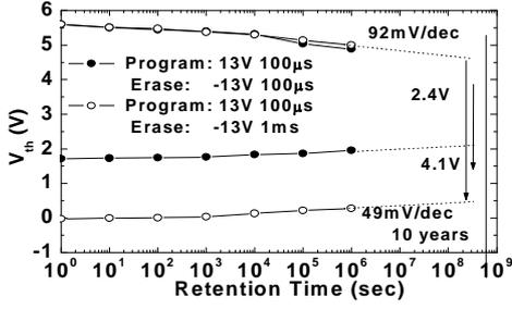
Fig.9. Retention of MONOS devices with 12nm AlN at 25°C
