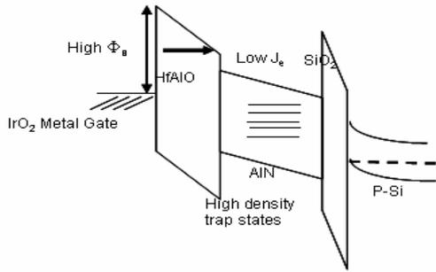
Fig.1. Band diagram of IrO<sub>2</sub>-HfAlO-AIN-SiO<sub>2</sub>-Si MONOS memory in erase state. The higher work-function IrO<sub>2</sub> allows thinner HfAlO w/o large electron injection into AIN.
