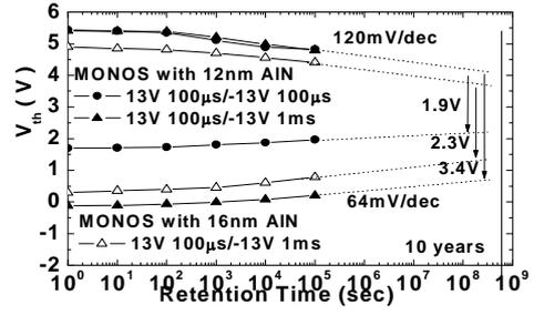
Fig.10. Retention of MONOS devices with 12nm and 16nm AlN
