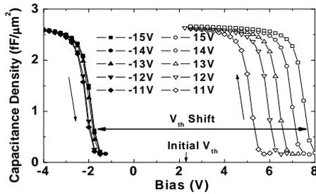
Fig.3. C-V hysteresis curves of MONOS capacitor with 16nm AIN for various  $V_g$ . The capacitance density increases to 3.5fF/ $\mu\text{m}^2$  for 12nm AIN device.
