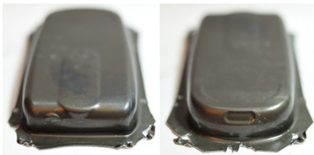
Fig. 38 Ti/Al clad metal housing without failure (holding force, 0.7 t; chamfer width, 20 mm)
