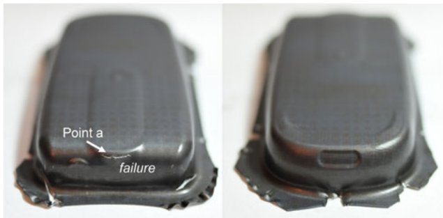
Fig. 37 Failure of the Ti/Al clad metal housing occurs at point a (holding force, 1 t; chamfer width, 20 mm)
