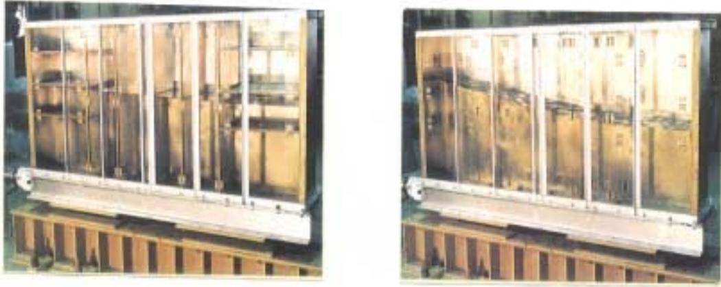
圖 1.3 Aqua Damper(Tuned Slushing Water Damper)
