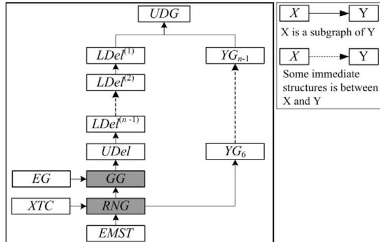
Fig. 2: The relations of the pure localizable structures and their extensions.
