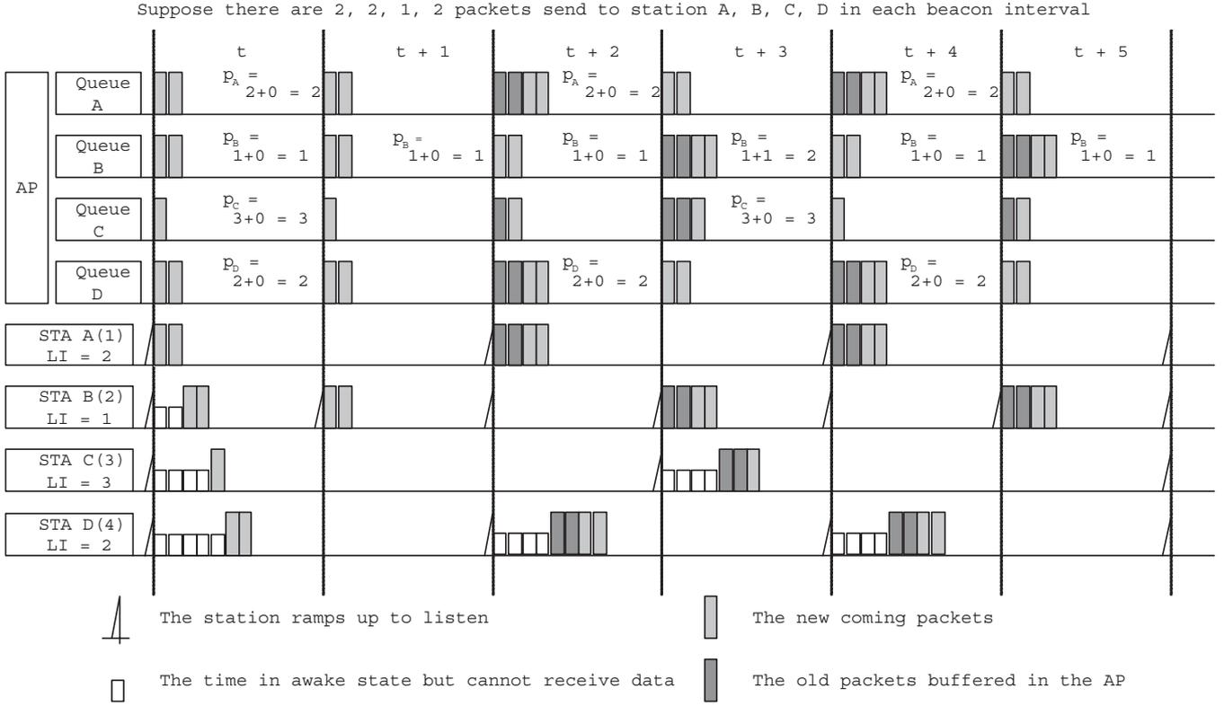
Figure 3: An example of the smallest AID first method
