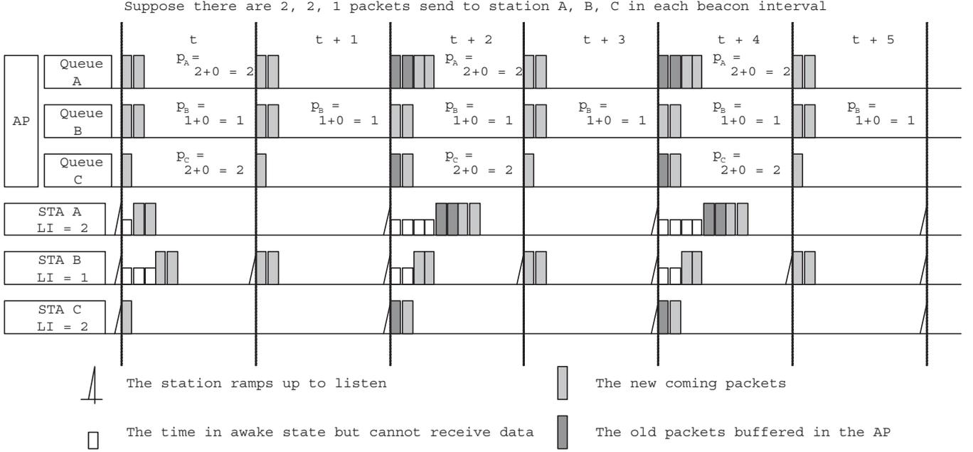
Figure 4: An example of the smallest queue length first method
