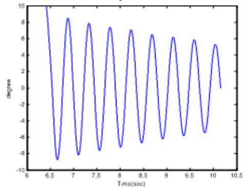
Figure 14. Trajectory of  $\theta_0$  to stabilize the pendulum with time delay = 0.019s
