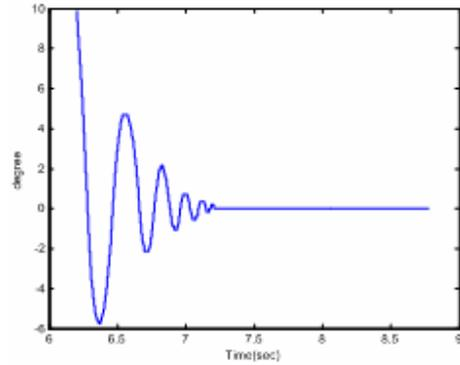
Figure 13. Trajectory of  $\theta_0$  during the stabilization of the pendulum
