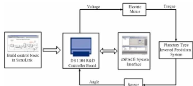
Figure 9. Overall hardware configuration using DS 1104
