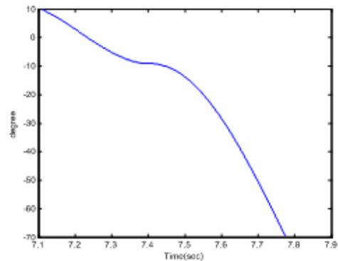
Figure 15. Trajectory of  $\theta_0$  to stabilize the pendulum with time delay = 0.020s
