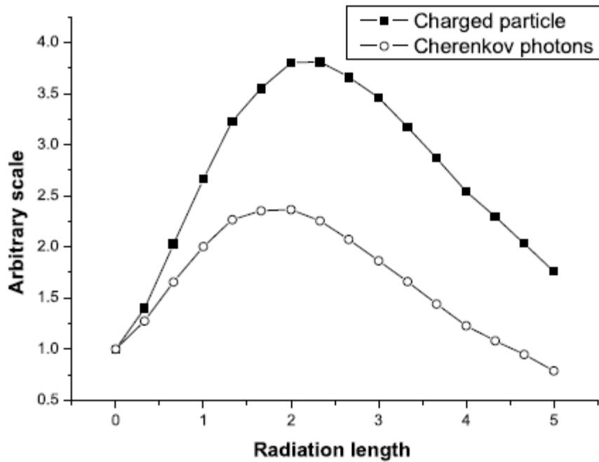
**Fig. 6 The longitudinal profile and Cherenkov photon yield as a function of radiation length.**
