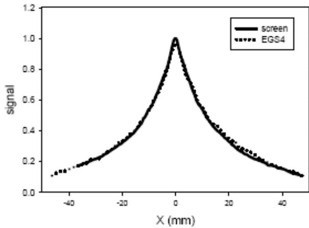
**Fig. 2 Shower spread at 10 radiation lengths, projected on to x-axis. Y-axis range is  $\pm 4.8$  cm**
