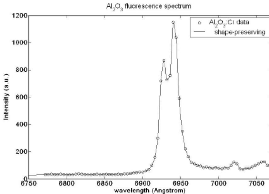
**Fig. 4 The fluorescence spectrum of  $\text{Al}_2\text{O}_3:\text{Cr}^{3+}$  scintillator. Two close peaks located at wavelengths 692.8 nm and 694.0 nm are clearly seen.**
