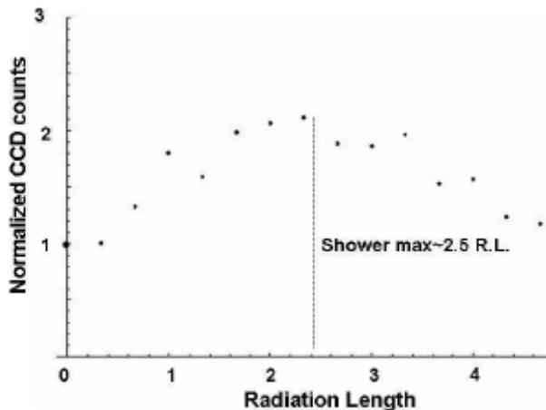
**Fig. 5 The shower longitudinal profile as recorded by the CCD camera.**
