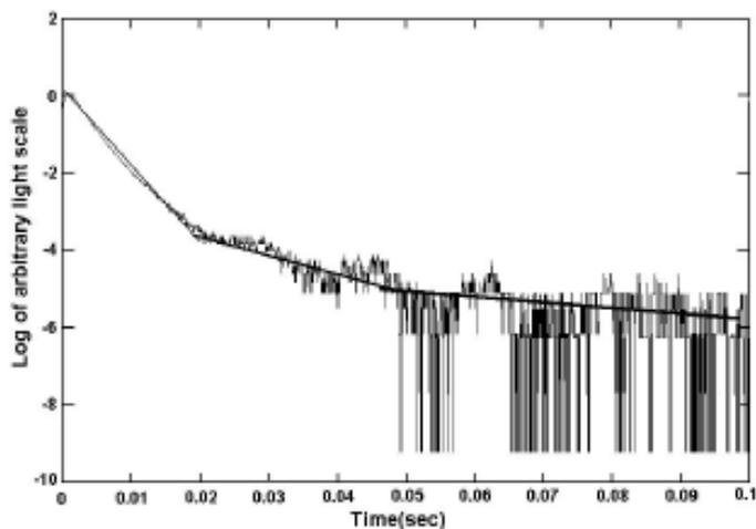
**Fig. 3 Results from the decay-time measurement. This decay-time of the scintillation light from  $(\text{Al}_2\text{O}_3:\text{Cr}^{3+})$  is measured by photo-diode and digital multi-meter. The first decay pattern has a decay time of 3.4 ms, the second one has a decay time of 6.7 ms and the third one has a decay time longer than 15 minutes.**
