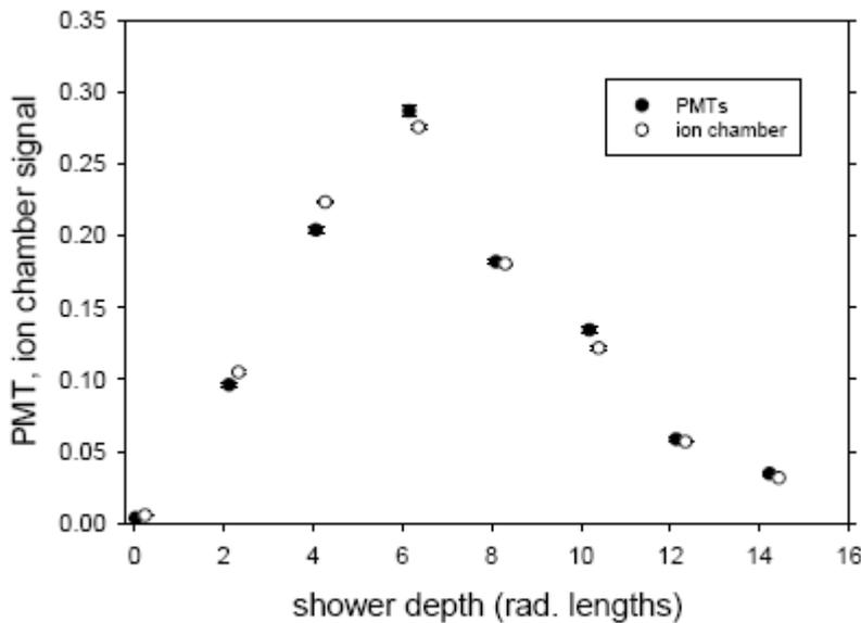
**Fig. 1 Comparison of fluorescence and ionization longitudinal profiles. The sums of their points are independently normalized to unity.**
