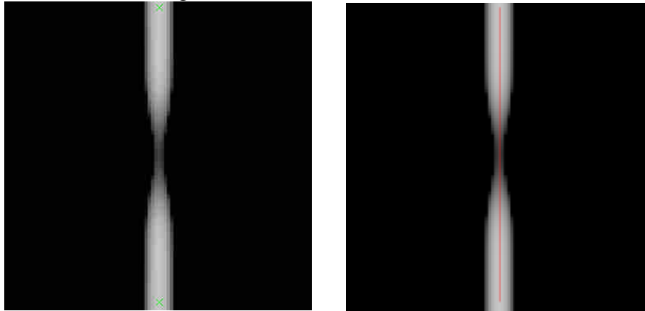
Figure 6: A computer generated phantom data set. The original image is shown on the left and the center line obtained is show on the right.
