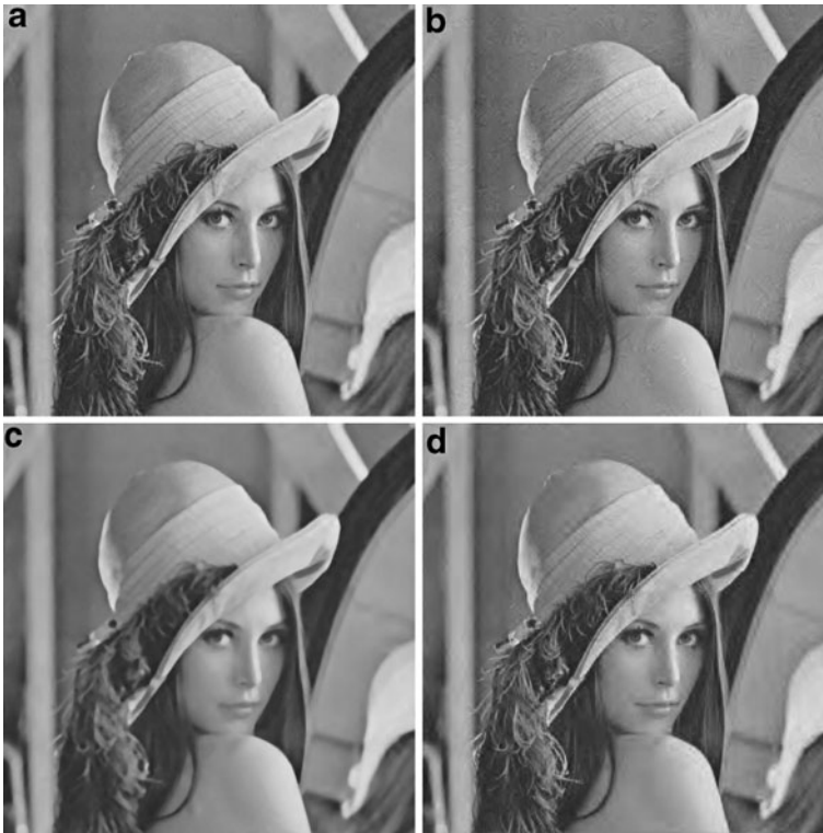
Fig. 4 a Original watermarked Lena image by DEED R b JPEG compressed Lena image with QF=40%, PSNR=33.49dB and \rho=1 c 4×4 Median Filter attacked Lena image with \rho=0.86 d The attacked Lena image where 5 lowest bitplanes in the wavelet domain are removed. PSNR=33.2dB, \rho=0.88
