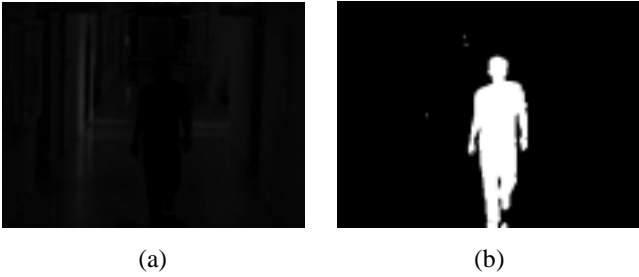
Fig. 1. (a) Difference between current frame and background image. (b) (a) is applied a threshold.
