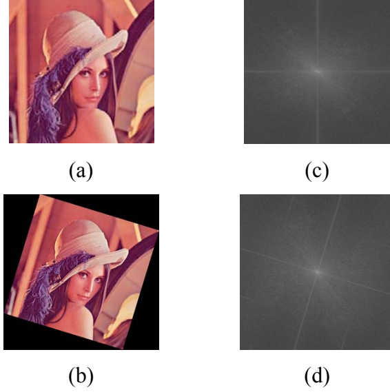
Figure 1 Input images, and Fourier spectrum images of G channel. (a) Image “Lena”. (b) Image “Lena” after rotation. (c) Fourier spectrum image of image “Lena” (d) Fourier spectrum image with the same rotation angle of (b).
