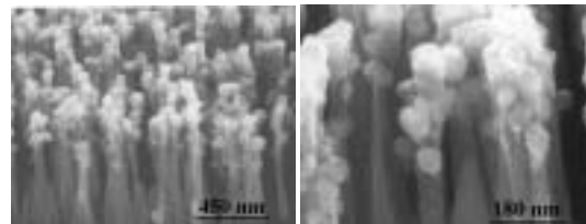
Fig. 3 (a) High and (b) low magnification of SEM photographs of DLC-clad Si nanotips.
