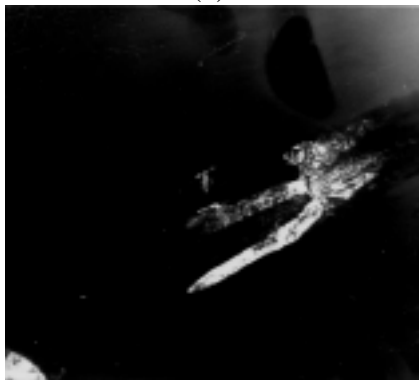
Fig. 7. (a) TEM bright-field image, (b) corresponding selected area diffraction pattern and (c) dark-field image of self-assembled ZnO bundles.
