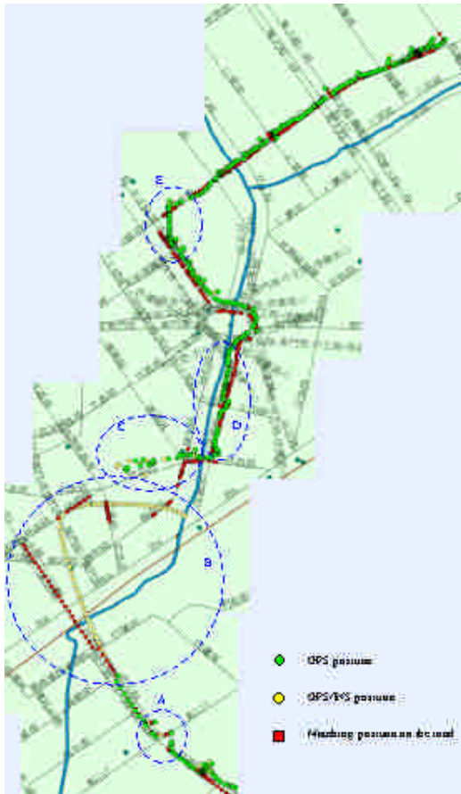
Figure 17 GPS/INS without the GIS correction
