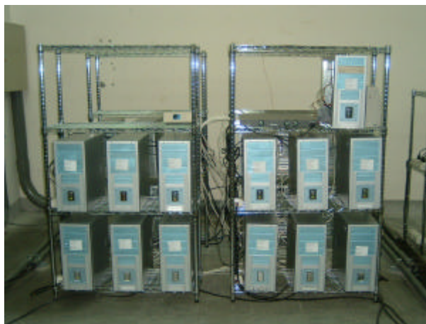
Fig. 2 23-node PC-Cluster system at MuST
