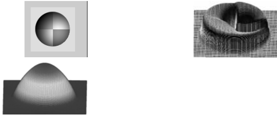
Fig. 2 (a) The image with different albedo on the same surface. (b) The reconstructed result by the conventional method. (c) The reconstructed result by the proposed method.
