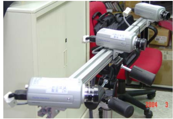
Fig. 6 Three cameras on the camera holder
