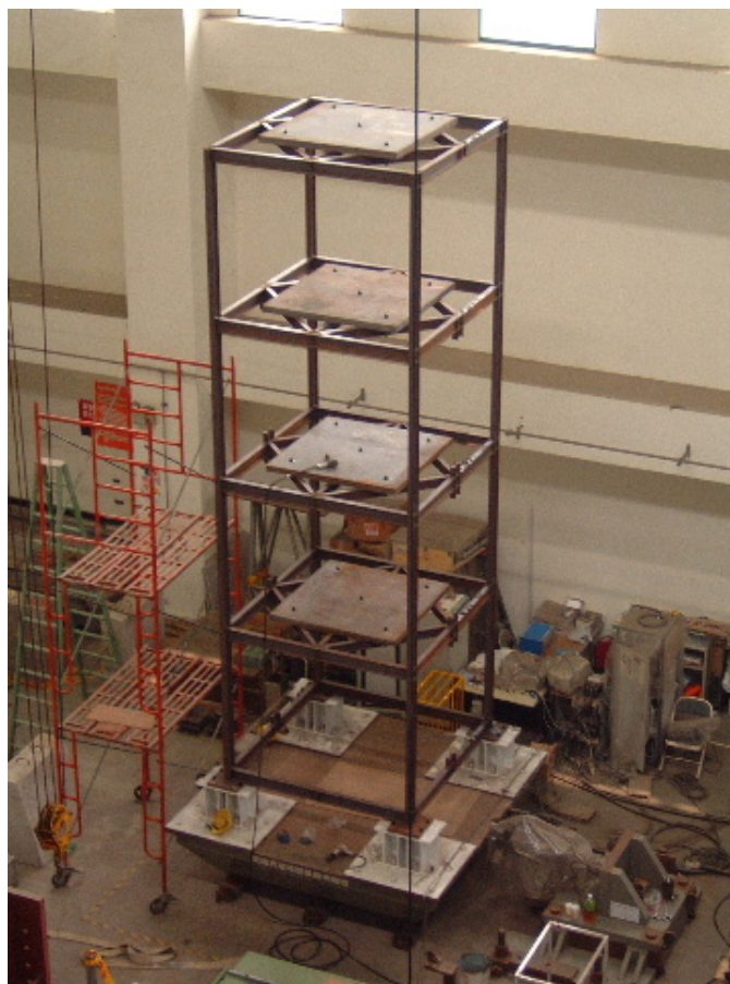
Figure 4.5 A photo of the four-story clear frame
