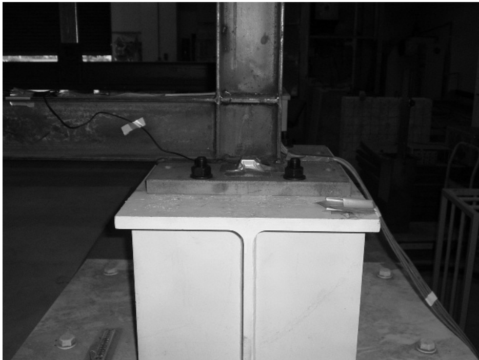
Figure 4.8 Accelerometer at the base of the test frame
