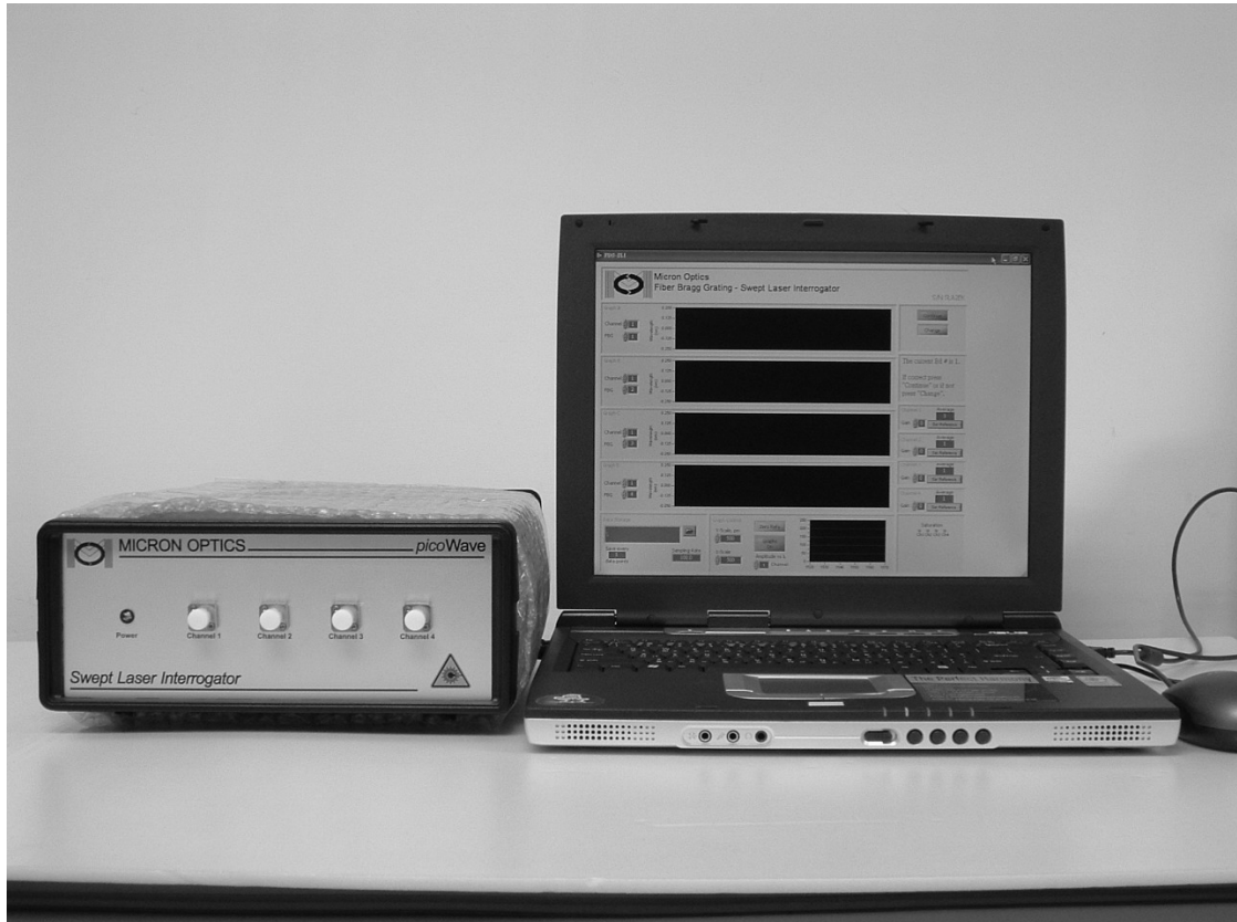
Figure 4.11 FBG data acquisition system
