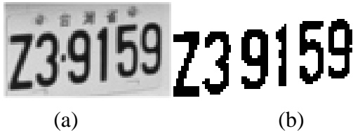
Fig. 10: (a) The license plate image of Fig. 7(a); (b) The binarized and de-noised result of (a).
