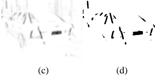
Fig. 7: (a) The car image with a license plate; (b) The vertical gradients of Fig. 7(a); (c) The local variance of Fig. 7(b); (d) The possible license plate regions.
