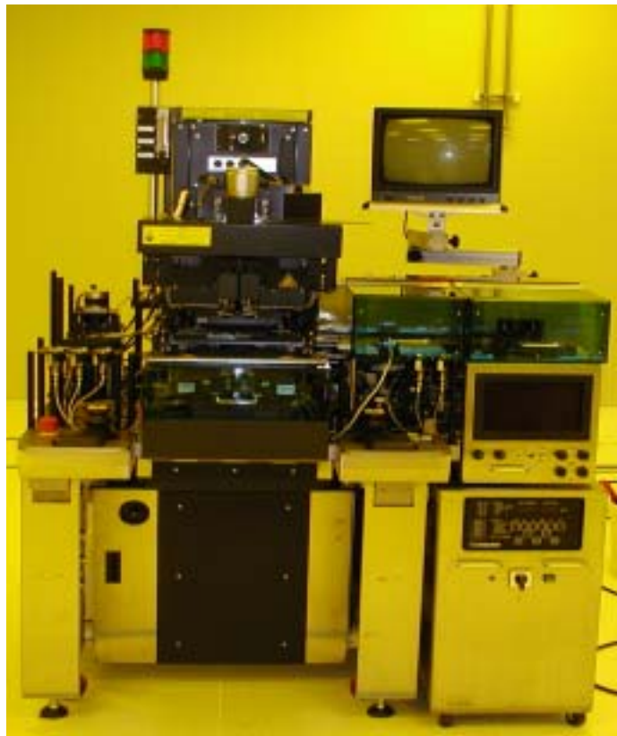
Figure 2 Mask Aligner SUSS MA 150CC
