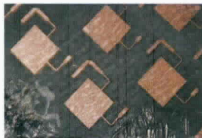
Fig 3.2-5 Picture of elements on the main reflector
