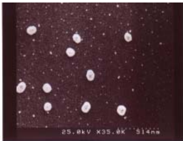
Fig.2 SEM picture of particles collected at tube wall.
