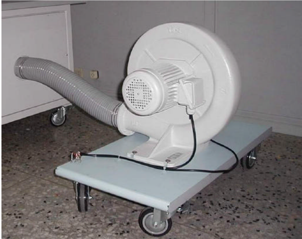
FIGURE 7 The connecting of blower and tunnel
