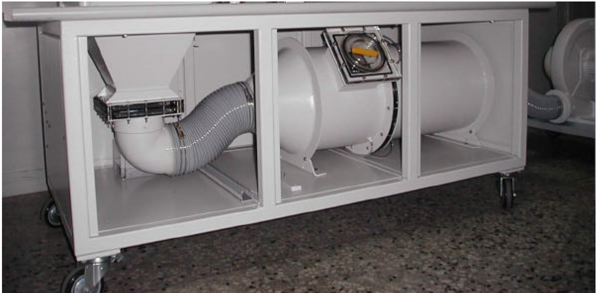
FIGURE 4 The picture of AMCA 210-85 standard in wind tunnel
