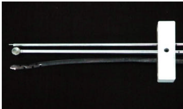
FIGURE 17 The picture of bi-directional pitot tube
