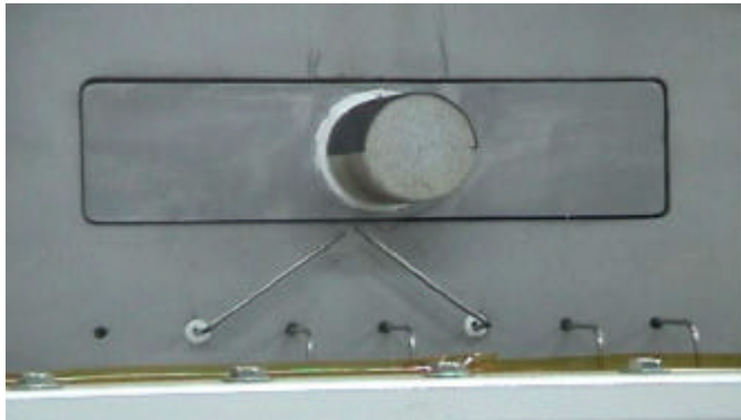
FIGURE 9 The pitot tube in test section
